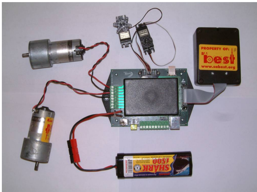
Figure 3. This is your first complete BRAIN test setup.
